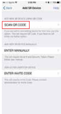
3 Tap SCAN QR CODE and scan code. *QR code is located on back of SR Ethernet bridge and front of this guide
